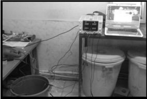
Figure 1 Acceleration corrosion setup
